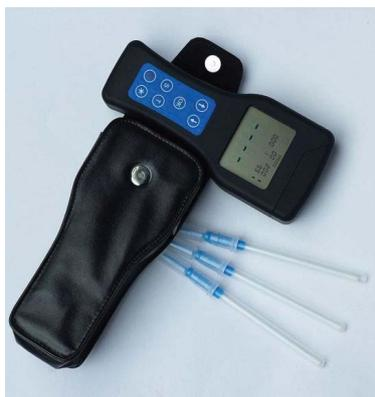
**Figure 8** luminometer used to detect bioluminescence.
